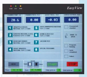
There are also two test programs which are: Bowie&Dick and vacuum leakage.
